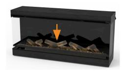
**14)** Carefully lift the AR front glass up and into the bottom front grooves of the appliance, then in at the top.
