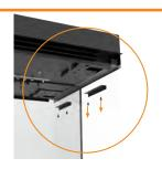
7) Remove the mirrored rear glass from rear of the appliance by carefully offering the bottom of the glass out at the bottom then the top.
