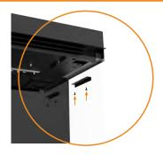
13) Carefully place the Deluxe fuel bed tray into position and ensure the fuel bed tray is back against the rear glass, so a gap is created at the front of the fuel bed.
