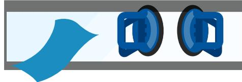
3. Open the handles of the suction cups and press them firmly onto the glass, ensure there are no air bubbles, then place the handles together on each suction cup. Ensure the cups are secure in position on the glass and lift.
