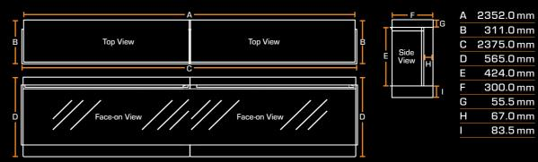
This model has two 1500w heaters which requires two 10 Amp outlets drawing a total of 13.05 Amps. Therefore, it may require it's own circuit. For an optimal installation, it is recommended that it is hardwired with it's own circuit.
